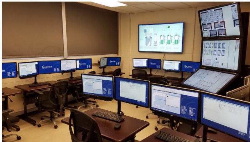
Figure 1. Simulator room showing the three vertically stacked touchscreen displays and connected computer systems.
